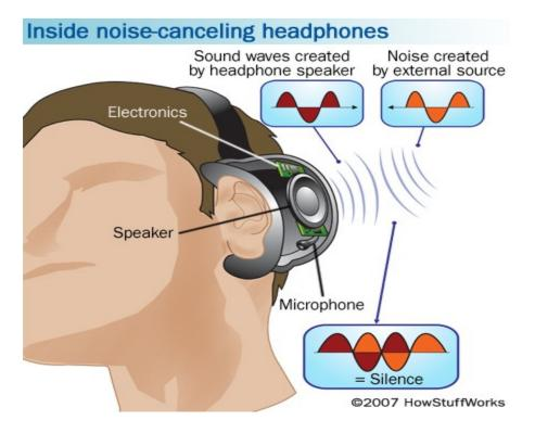
The headphones that are on the consumer market today which do use ANVC technology are only able to drone out low frequency waveforms and not high frequency ones thus relying on the passive or structural nature of the earphones to aid in eliminating high frequency. There are a few reasons for this first is that it simplifies the electronic circuitry, and second active cancellation is not as effective at higher frequencies since higher frequency waveforms have a shorter wavelength.
