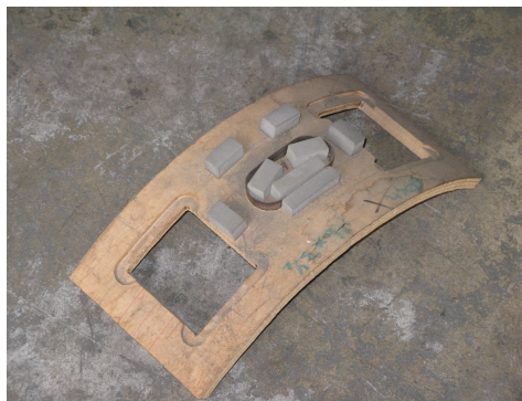
Example of a Partial Die, a Hand Hole
