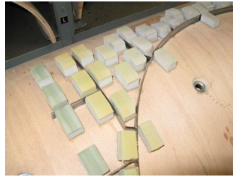
Die Rubbing and Steel Rule
